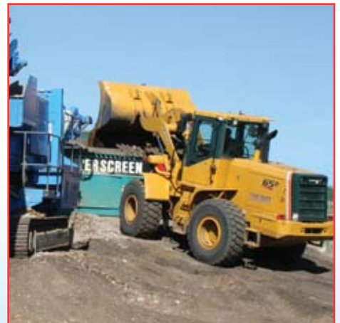
This 65ZV-2 feeds rainbow rock to a crusher to begin the multi-step process of pulverizing the material fine enough to merit its name.
